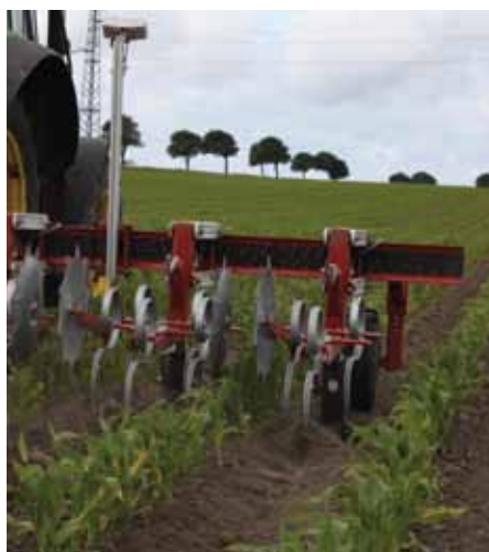
Camera steering allows higher speed, thus increased capacity.
