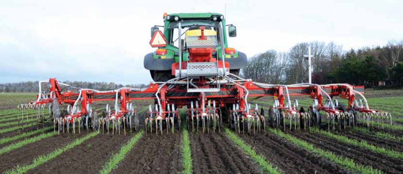
VCOF 8-75 with section control – outer section to the left is raised.
