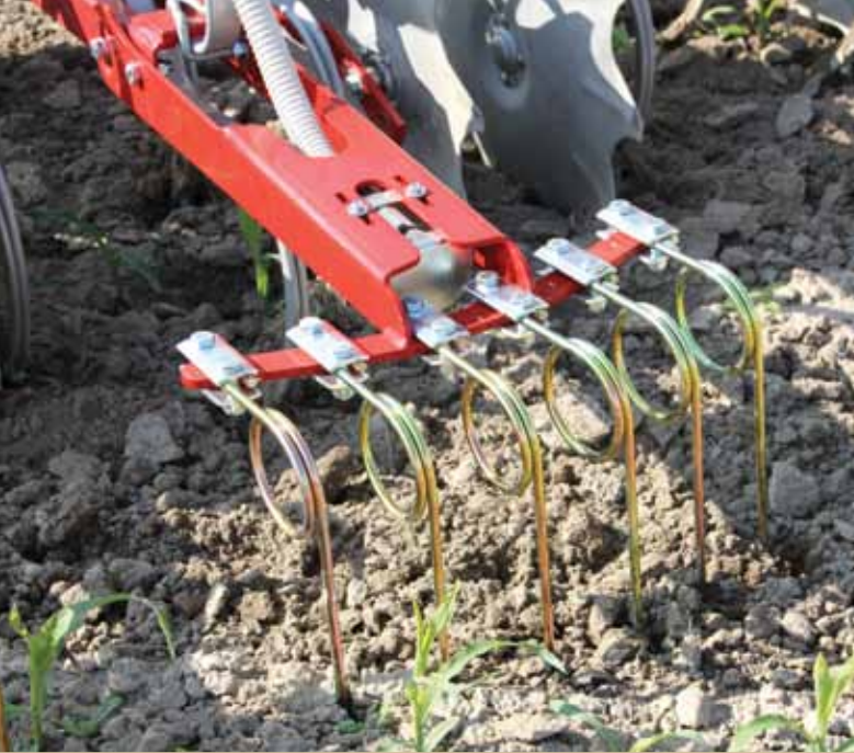
Simple and sturdy rear harrow protecting FS Seeder spreader plates.
