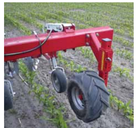
Large tractor pattern support wheels ensure a stable and accurate beam position.
