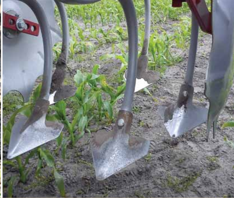
Cleaning sections with genuine Kongskilde fines and shares and rotating plant protection shields for optimum cleaning.
