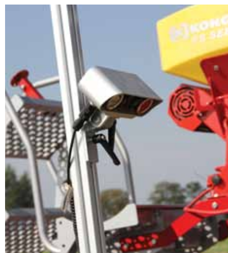
The height and angle of the stereo camera can be adjusted depending on the actual growth stage of the crop.
